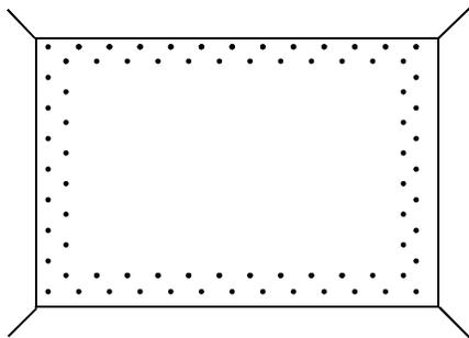
Figure 10: Drilling masonry for Deepflow/ Deepwood
