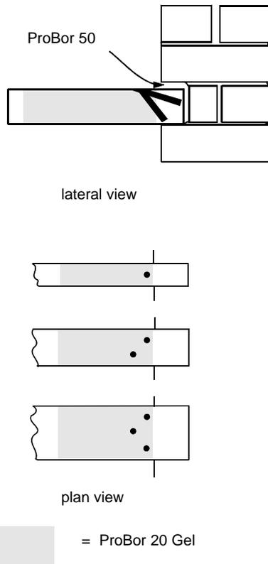
ProBor 20 Gel is supplied in 25 litre containers. It is a moderately viscous liquid which can be applied by brush and by dipping.
