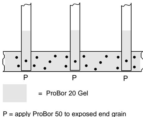
Figure 13: Joists on sleeper walls
