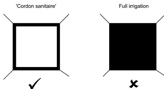
(‘toxic box’) could be used (Fig. 6) This involves drilling perimeter of the infected area and injecting masonry sterilant into the masonry under pressure; the work is finished with a liberal surface spray or brush treatment with the sterilant
