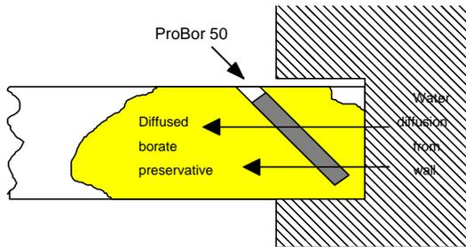
Like the borate rod Safeguard ProBor preservatives are water soluble and will readily diffuse into damp wood, even from the surface. But unlike the rods diffusion is significantly more rapid and efficient because the material is supplied as a water miscible liquid/paste. The glycol in which the borate is dissolved and suspended is hygroscopic thereby causing rapid mixing of the soluble borate with any resident moisture.
