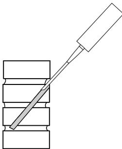
Where the whole length of a wallplate is embedded then drill a staggered pattern of 8 - 10mm diameter holes broadly as shown in Figure 12.
