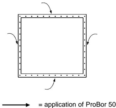
Figure 16: ProBor 50 applied to masonry
